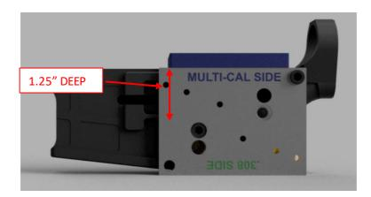
**Step 5:** NEXT ROTATE ITEM 3 OR TOP ROUTER/MILL PLATE 180 DEGREES AND INSTALL SCREWS AGAIN. PLEASE SEE IMAGE BELOW.
