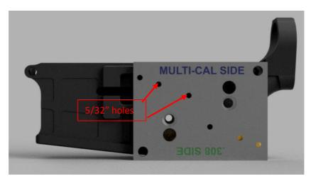
**Step 13:** DRILL OUT 3/8" SAFETY SELECTOR HOLE. BE SURE PART IS LEVEL IN VISE AND DRILL ALL THE WAY THROUGH LOWER RECEIVER (IT IS OK IF YOU DRILL INTO OTHER SIDE PLATE ). PLEASE SEE IMAGE BELOW.
